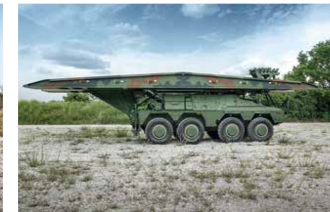
14 meter bridge LEGUAN MLC80/100
